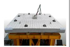
Punching shear in LCA slabs
